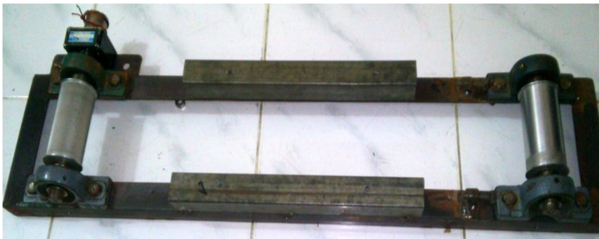
Figure 4.3: Steel panel with fixed roller & horizontally adjustable roller
