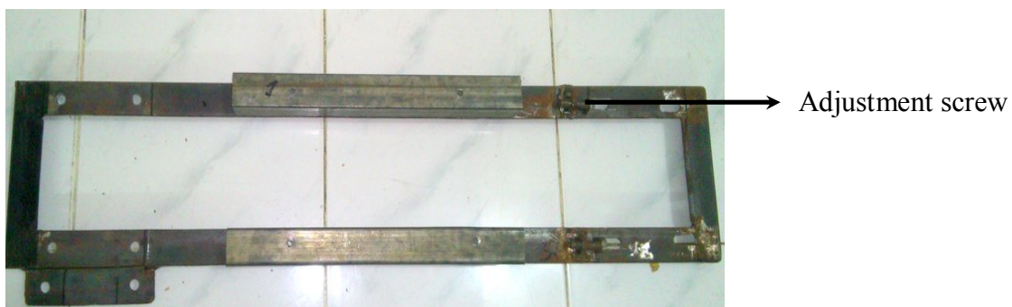
Figure 2.5: Steel panel structure
