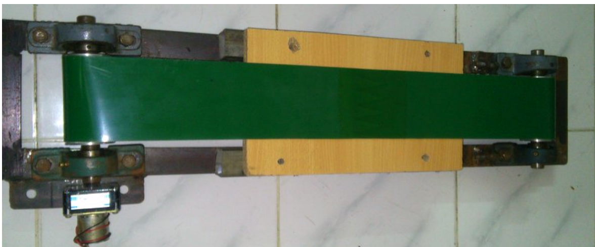
Figure 4.4: The complete conveyor belt with elements
