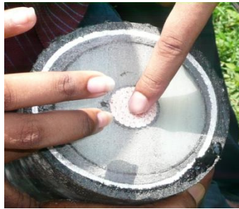
Figure 4.13: Underground Cable for 132kv Line
