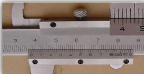
Figure 3.3: Vernier Calipers (Shimadzu, Japan)
