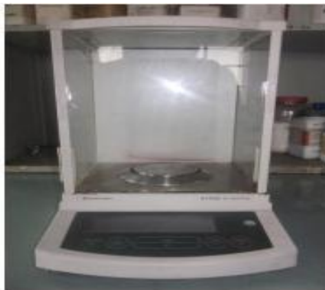
Figure 3.1: Analytical Balance (AY220, Shimadzu, Japan)
