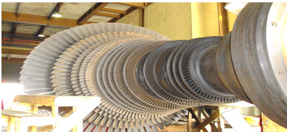
Figure 2.4: High pressure steam turbine
