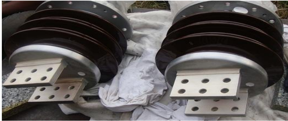
Figure 4.4: Bushing of a transformer [Source: Author]
