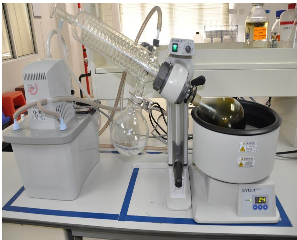
Figure 3.1: Drying of extract using rotary evaporator
