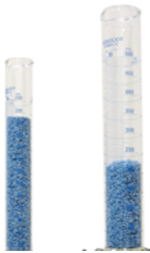
Figure 1.2: Bulk volume measurement without tapping and Tapped volume measurement after tapping (Anon, 2010)
