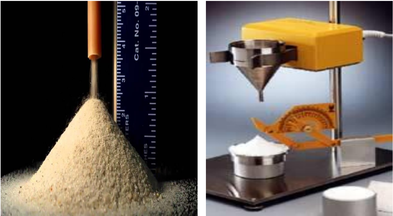
Figure 1.2: [Left to right] Measuring angle of repose and a set up of funnel
