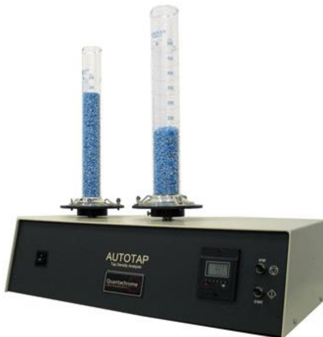
Fig 1.3: Bulk volume measurement without tapping (A) and Tapped volume measurement after tapping (B)
