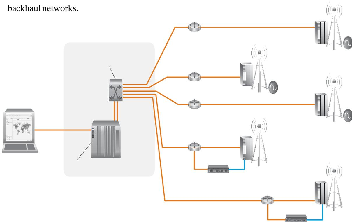
Figure 7.1: IEEE 1588 (PTP) Grandmaster Server Cards provide synchronization traceability over Ethernet to PTP clocks in remote base station.
