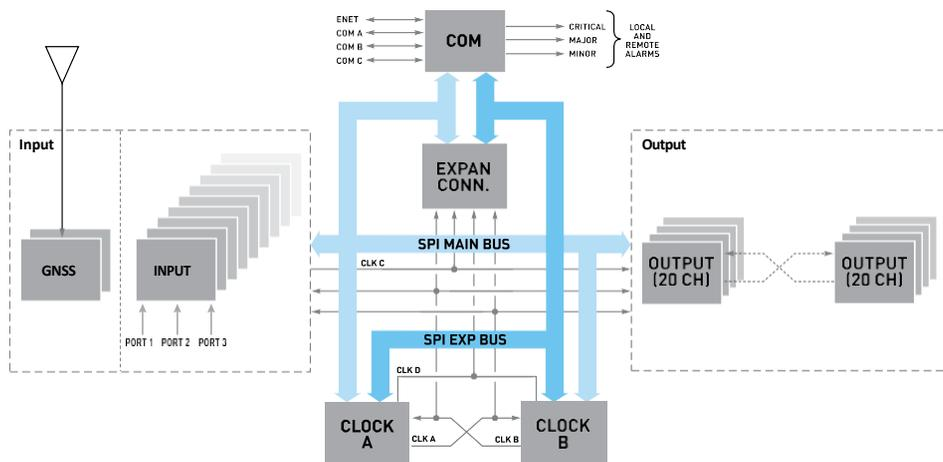
Figure 5.2: SSU 2000/2000e block Diagram
