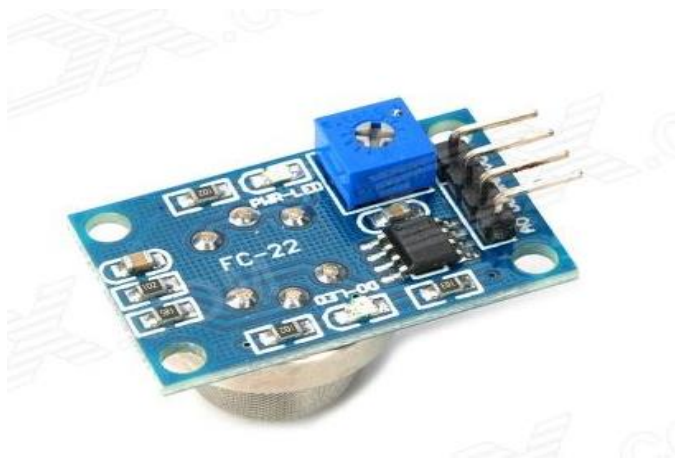
Figure 1.2: Smoke sensor FC-22
