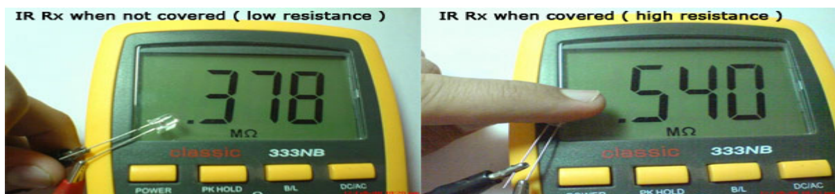
Figure 3.5: IR receiver (RX) is connected with multimeter
