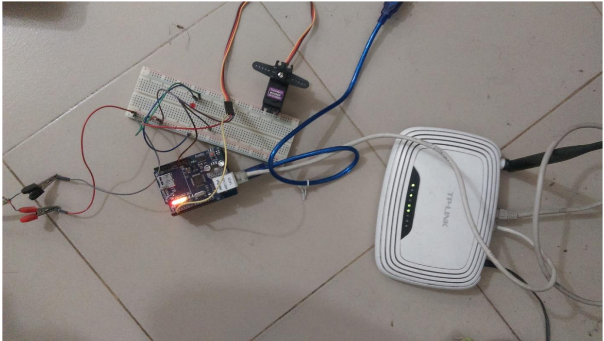
Fig 5.2: Connection with servo (servo on)
