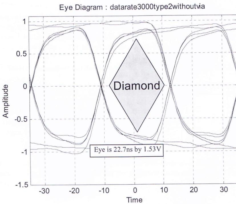
Figure 19: Eye diagram of Design type 2 without via at 3GHZ.
