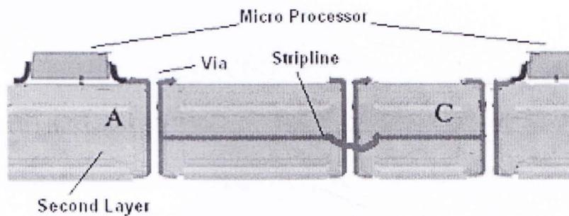
Figure 6: Configuration of system being analyzed (Side View)
