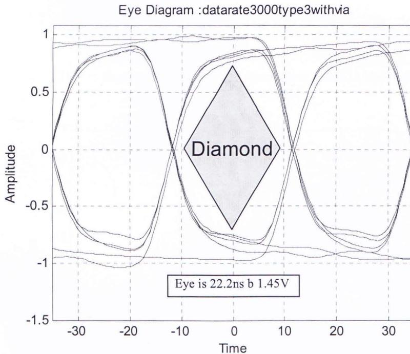
Figure 28: Eye diagram of Design type 3 with via & data rate is 3 GHZ. T-line is 13" long.
