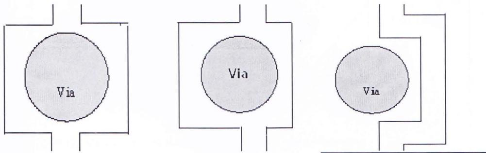
Figure 14: Via configurations, left - type 1, center – type 2, right - type 3.
