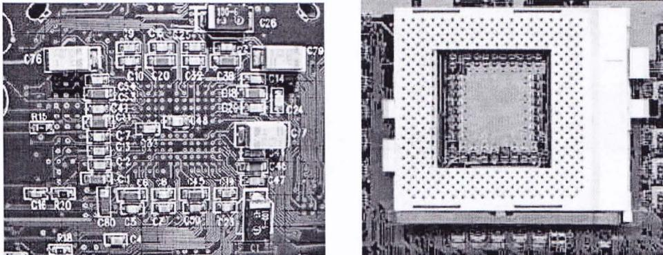
Figure 16: Surface mounted components and a CPU Socket of a Printed circuit board
