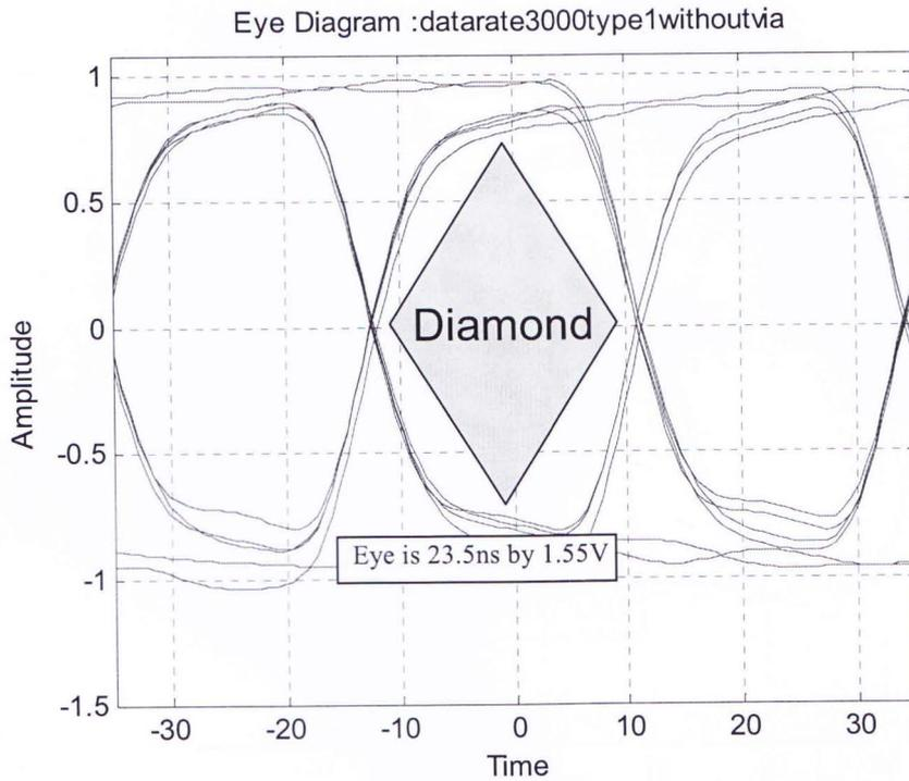
Figure 18: Eye diagram of Design type 1 without via at 3GHZ.
