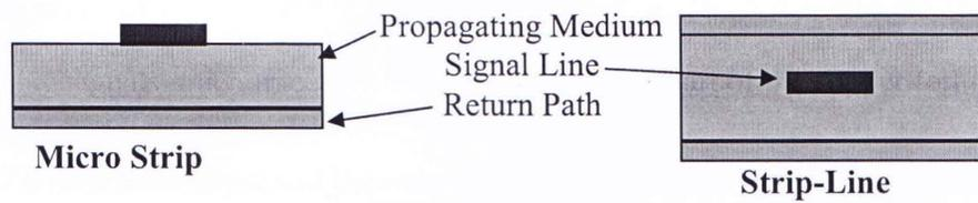
Figure 17: Microstrip (left, above) and Strip Line (right, above) configuration of transmission lines
