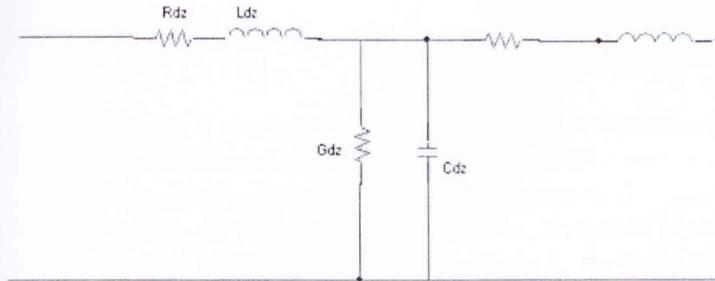
Figure 1: Discretized Transmission Line T-Equivalent Circuit
