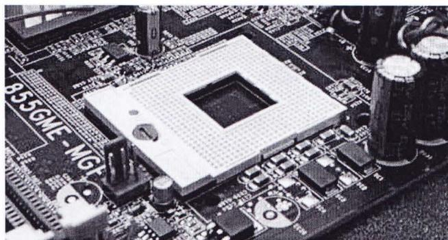
Figure 9: Socket on a printed circuit board.
