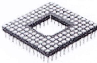
Figure 8: PGA type package
