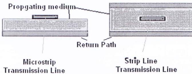
Figure 10: Types of Transmission Line
