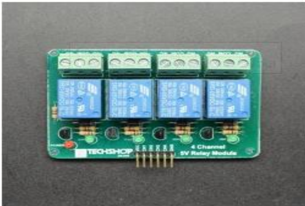
Figure 3: 4-Channel 5V relay
