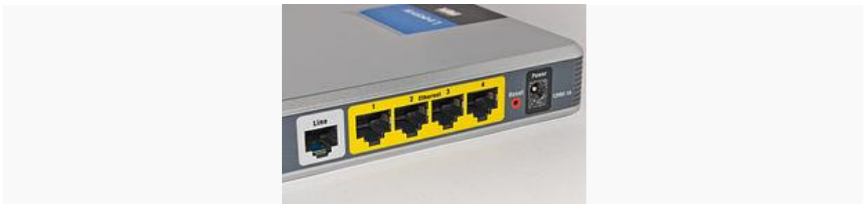
Fig.3.18.4 A typical home or small office router showing the ADSL telephone line and Ethernet network cable connections
