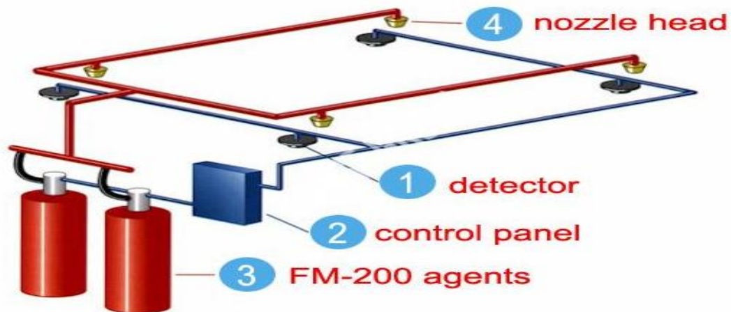
Figure 10.1: FM-200 fire suppression system.
