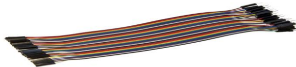
Figure 2.13: Male to Female Jumper
