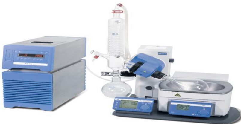
Figure 3.1: Drying of extract using rotary evaporator
