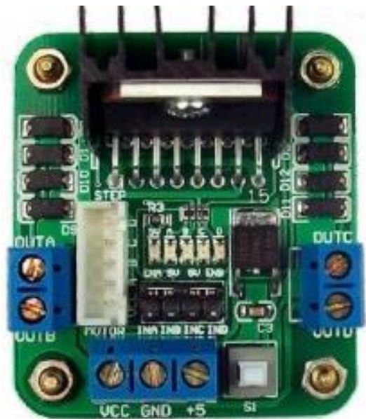
Figure 3.11: L298 Motor Driver [23].
