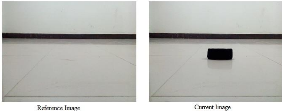
Figure 2.4: Example of typical reference image and image taken when object is present
