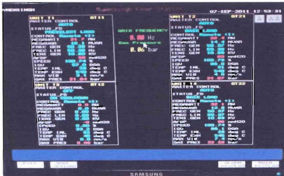
Figure 5.4: MARK-V using in MPS
