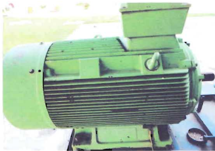
Figure 2.5: Induction Motor of MPS
