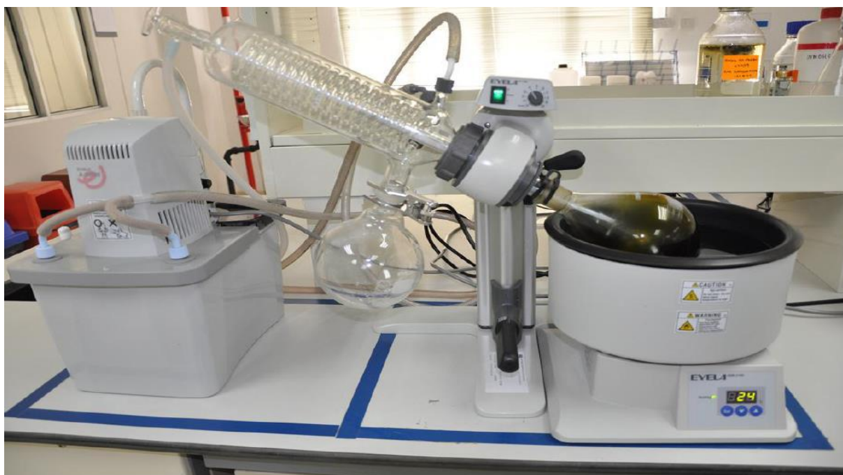
Figure 3.1: Drying of extract using Rotary evaporator
