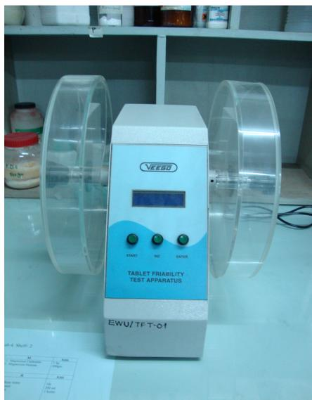
Figure 2.2: Tablet friability test apparatus.
