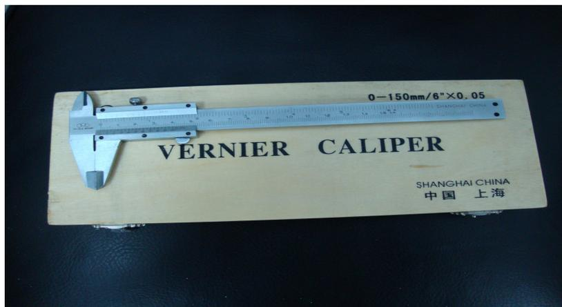
Figure 2.3: Vernier caliper
