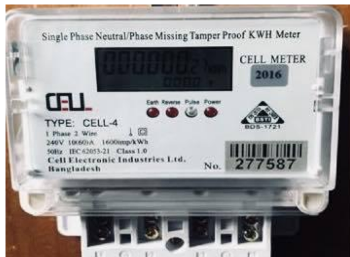
Fig 7.2: Single Phase Energy Meter (digital)
