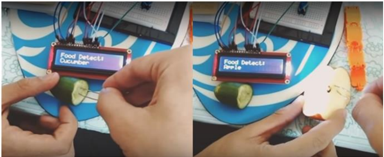
Fig 5.3: Apple and Cucumber detected by the device.
